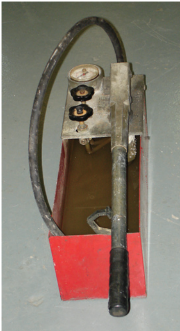
Figure 8.47 Example of a hydraulic test pump
