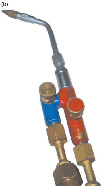
Figure 10.3 (a) Internal corner (b) tool for use in lead sheet bossing (Reproduced with permission of Lead Sheet Association)
