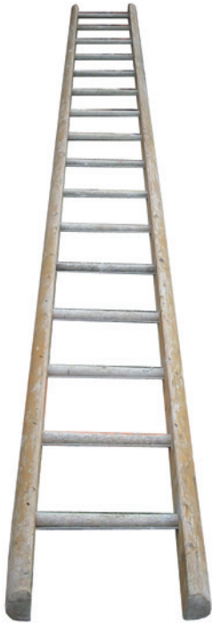
Figure 2.19 Typical wooden site ladder
