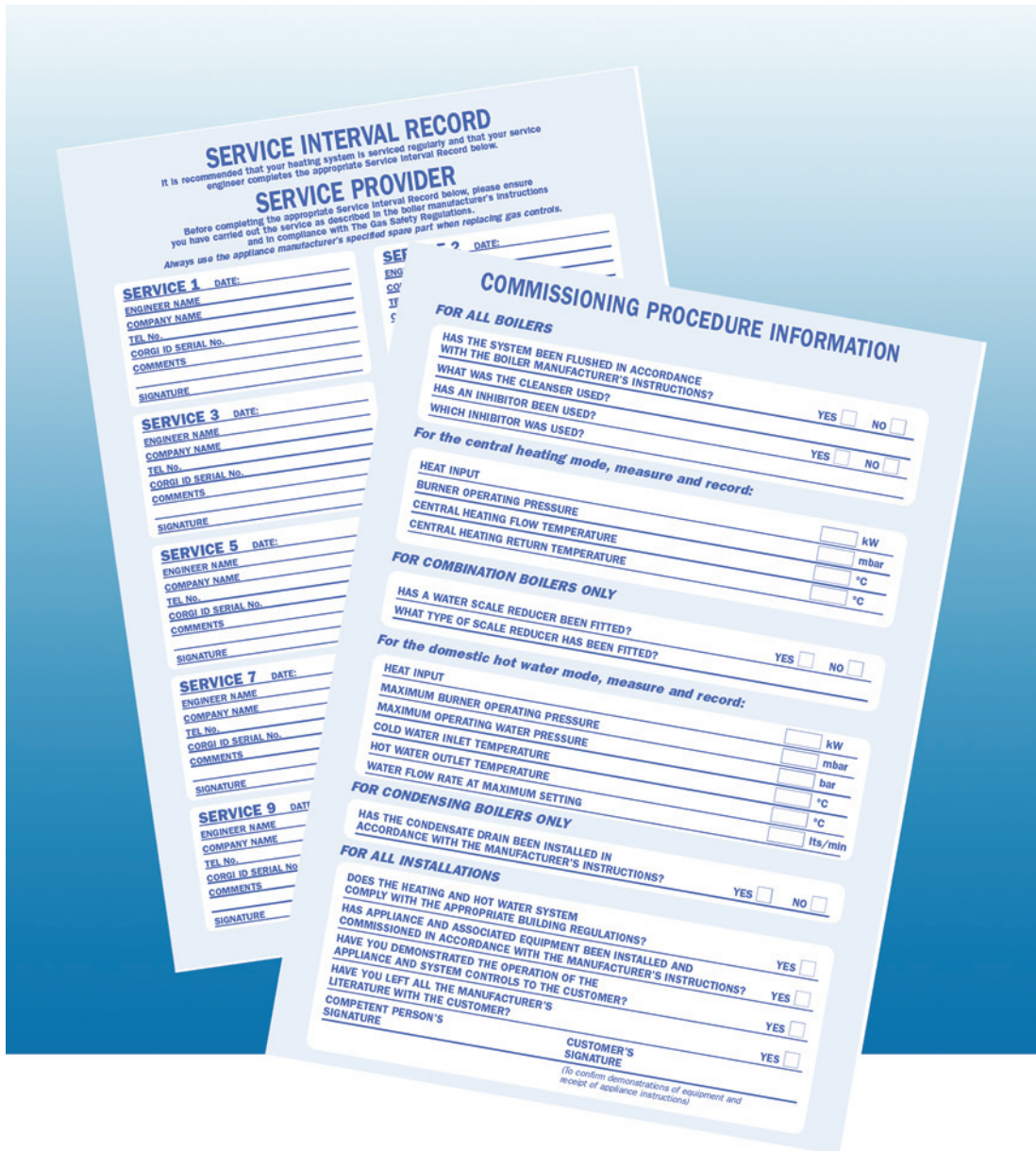
Figure 8.5 Benchmark service record and commissioning checklist
