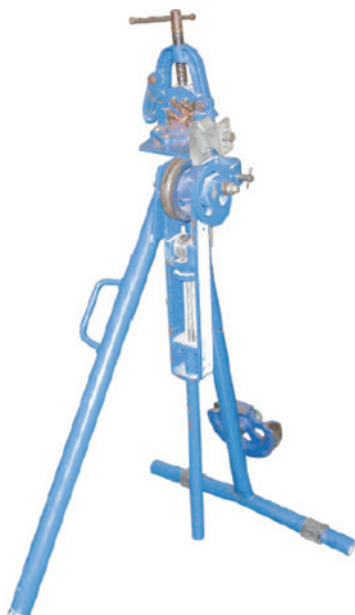
Figure 3.13 Free-standing pipe benders
